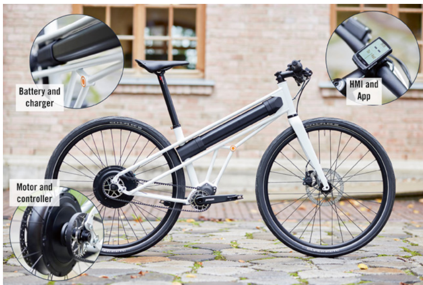
FIGURE 4 E-bike drive system (HMI: Human Machine Interface) (© Hirschvogel)
