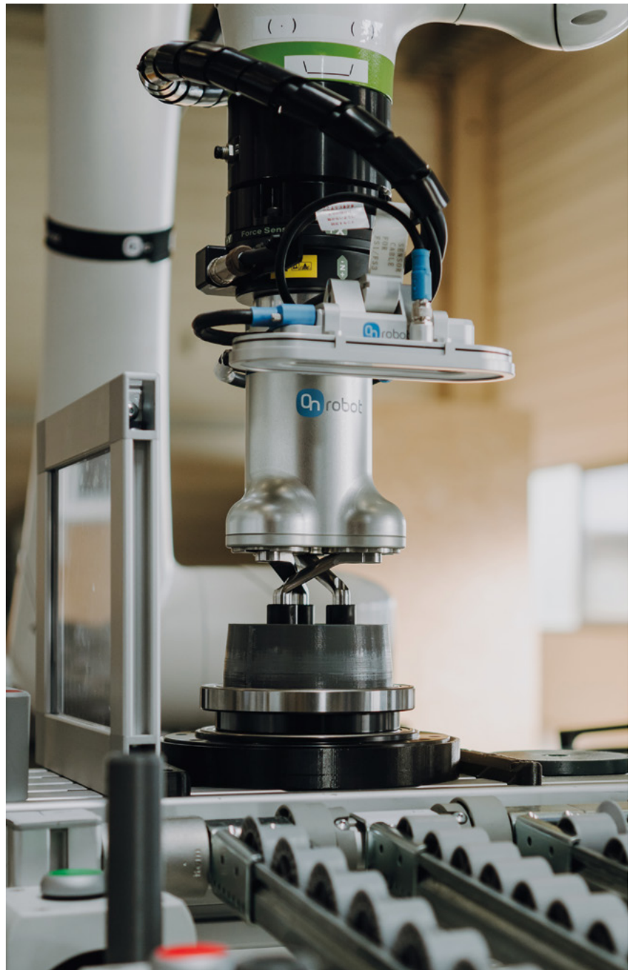
FIGURE 2 Collaborative robot (Cobot) (© Hirschvogel)
